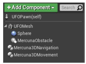
On any mesh or collision components on the pawn, under their Collision properties, ensure that "Can Ever Affect Navigation" is unchecked (this stops the pawn being considered as a static object in the navigation octree)
