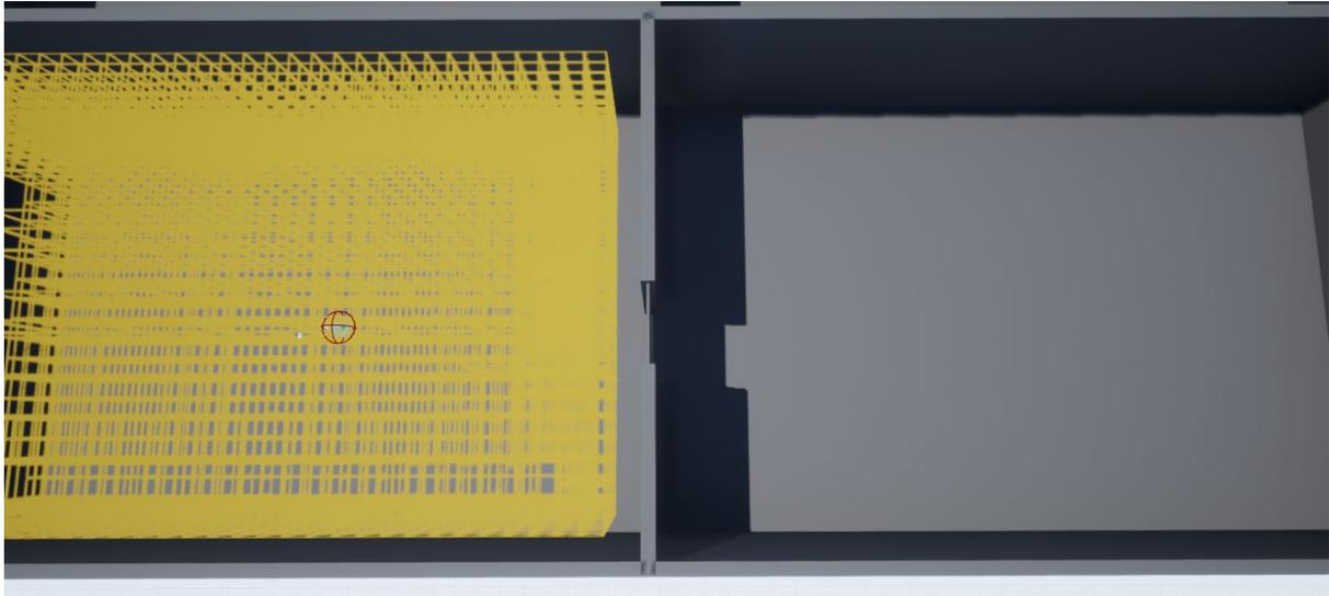
In the screenshot above, the yellow region on the left is navigable and seeded. The wall in the centre has a door in it, and when this opens Rebuild Volume is triggered through blueprint to regenerate the navigation data around the door.
