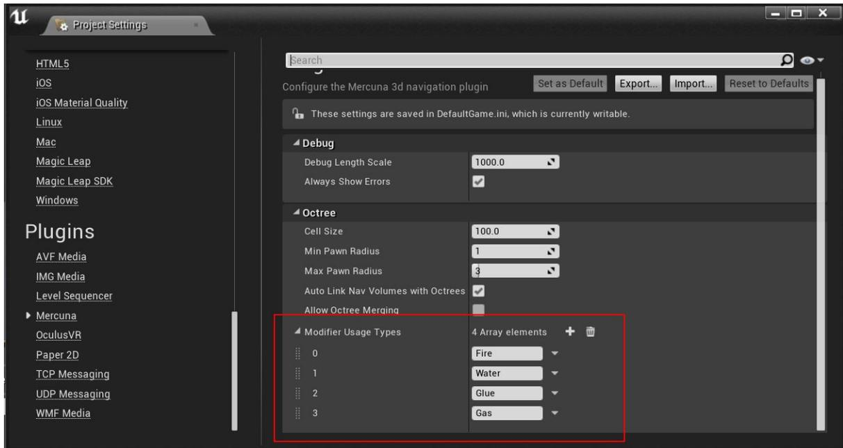
**Warning:** removing usage types, doesn't update the usage flags configured on existing modifier volumes or navigation components. Removing the Water usage type in the above example, means that all the usage flags on actors that previously corresponded to Water, will now be applied to the Glue usage type instead.
