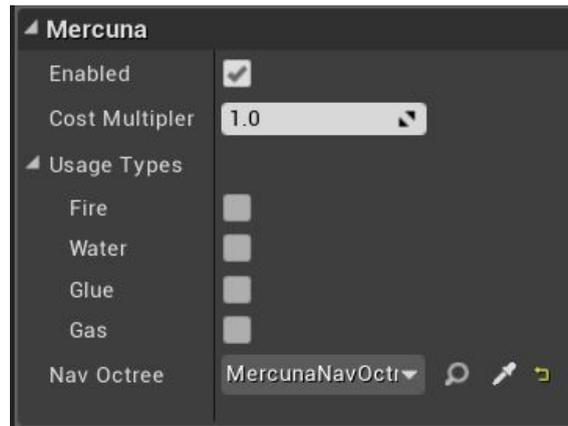
Whenever a volume is created, moved or resized in the Editor the navigation octree must be rebuilt for the change to be applied. Updating the usage types, cost multiplier or enabled setting does not require an octree rebuild.
